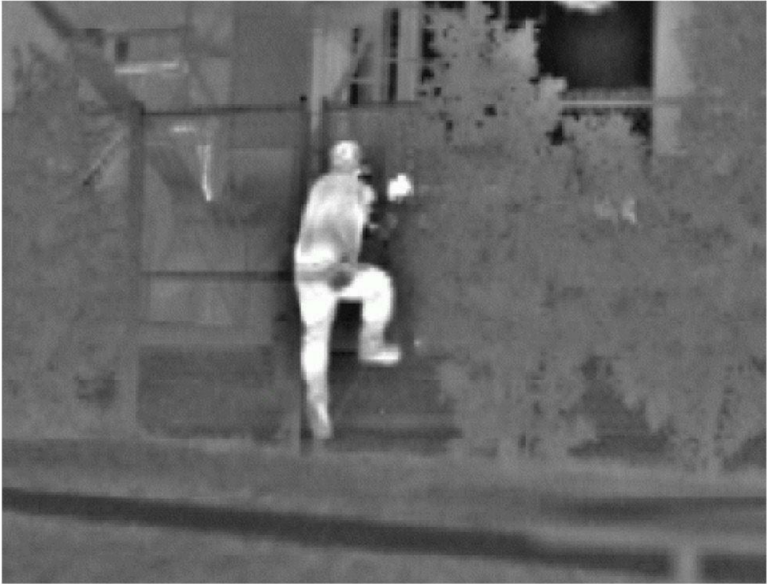
Figure 10.11 - An infrared camera is extremely effective in low-light areas and can provide the monitoring guard the ability to see in the dark
