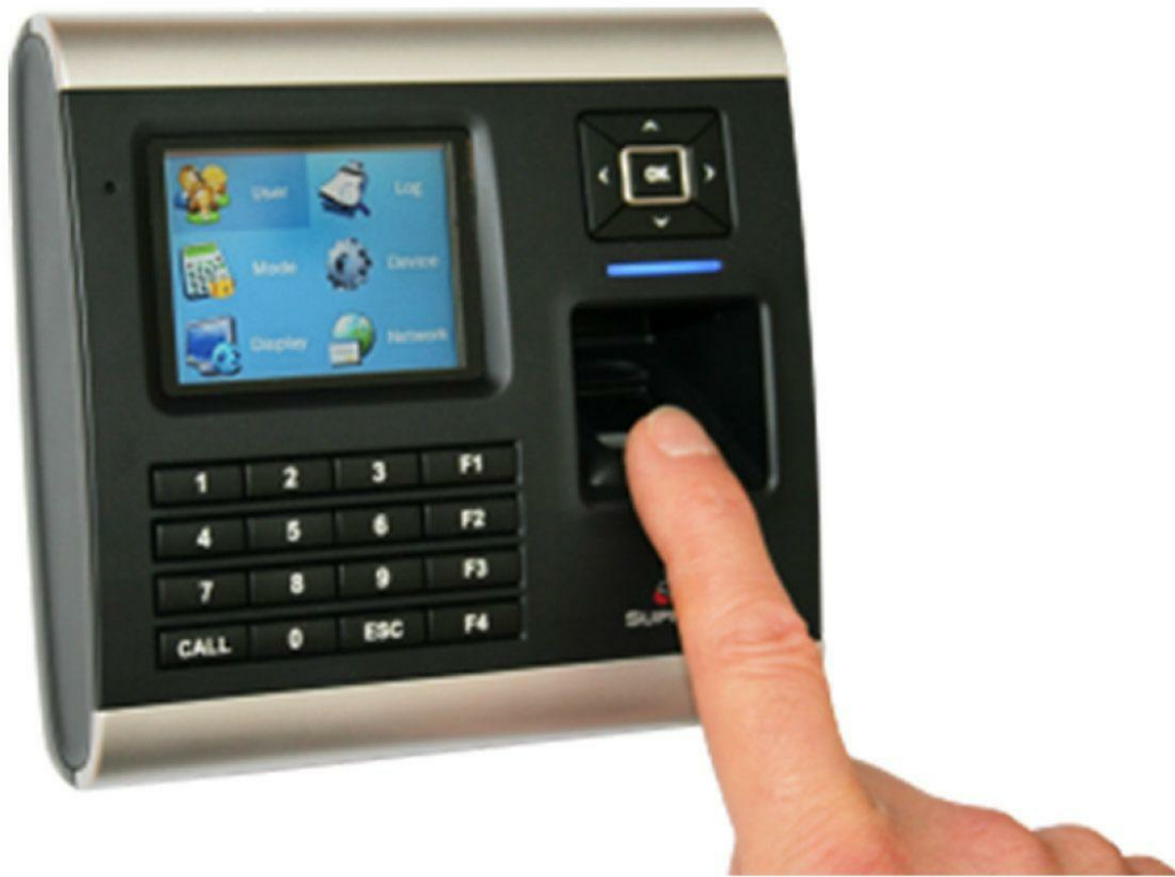
Figure 10.33 - A Fingerprint Reader scans the loops, whorls, and other characteristics of a fingerprint and compares it with stored templates. When a match is found, access is granted
