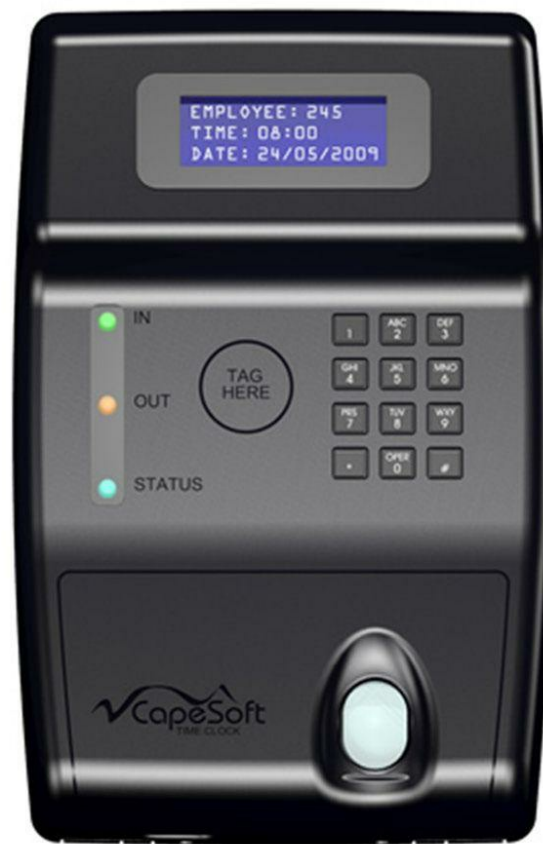
Figure 10.34 - A Card Reader with PIN and biometric features for additional security
