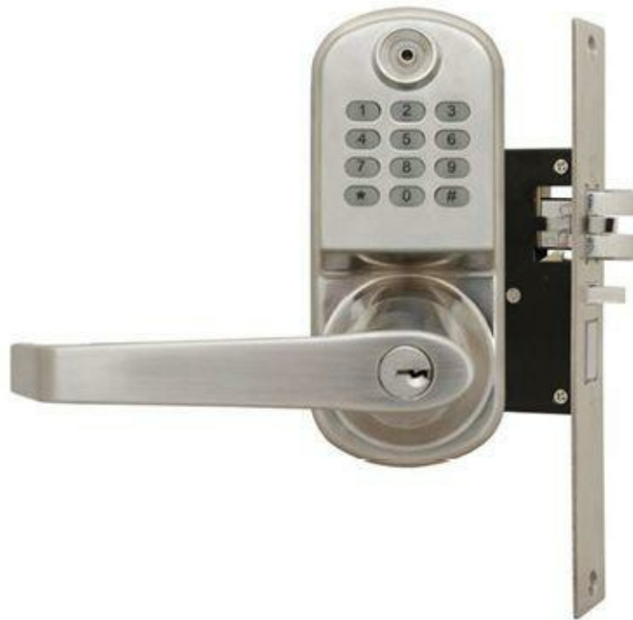
Figure 10.29 - A Ciper Lock is controlled by a mechanical key pad with digits that when pushed in the right combination will release the lock and allow entry
