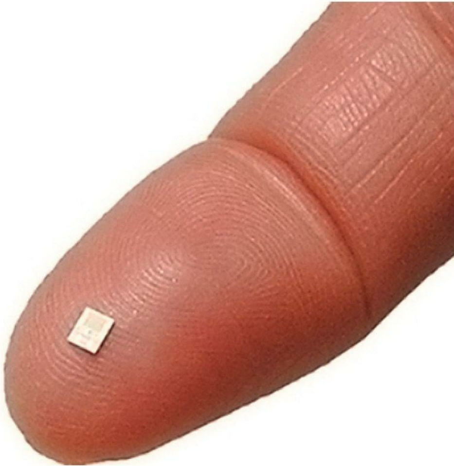
Figure 10.38 - Small and inexpensive Passive RFID tags
