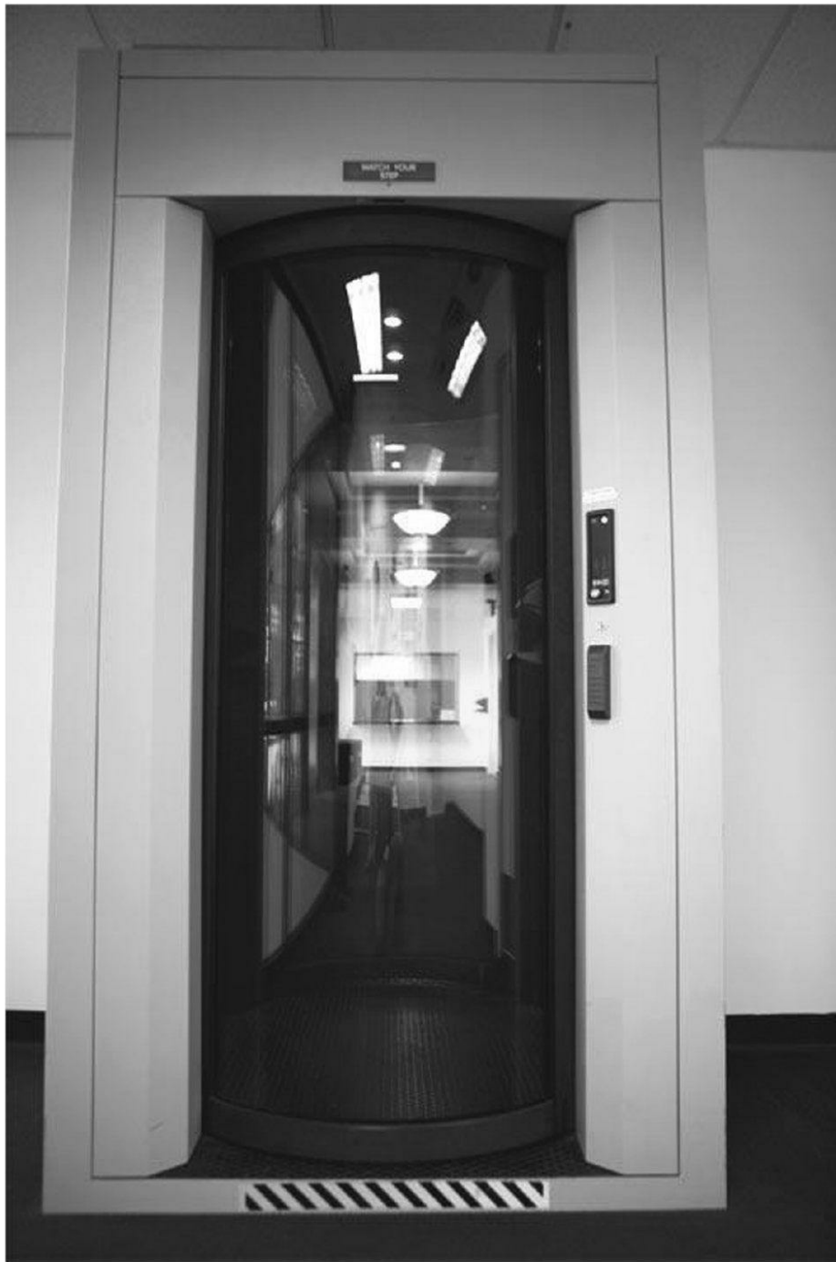
Figure 10.35 - A Secure Portal allows only one person in at a time and will only open the inner door once the outer door is closed (Courtesy of Bosch Security Systems)
